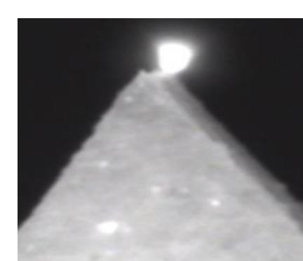
Figure 2. Corona discharge in PS-MS.
